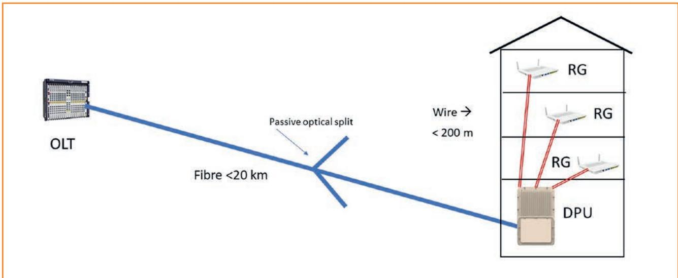
Figure 4: Fibre serving customers in Multiple Dwelling Unit (MDU)
