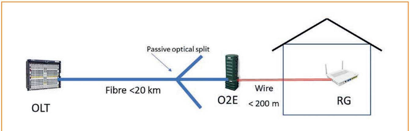
Figure 2: Fibre to the extension point for one home
