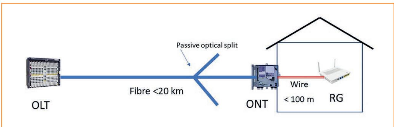
Figure 1: Fibre To The Premises (FTTP)
