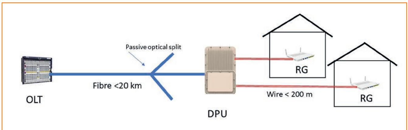
Figure 3: Fibre to the extension point serving multiple homes
