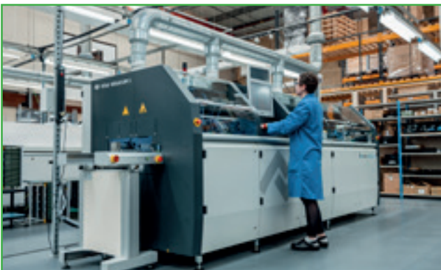
Celab's new Ersaflo selective solder machine
