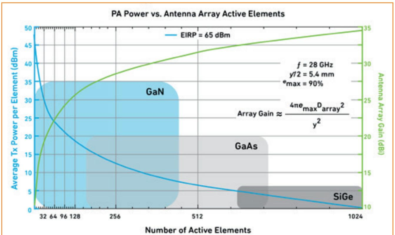
Figure 4: Trade-offs between the number of Antenna Array elements and RFFE process technology
