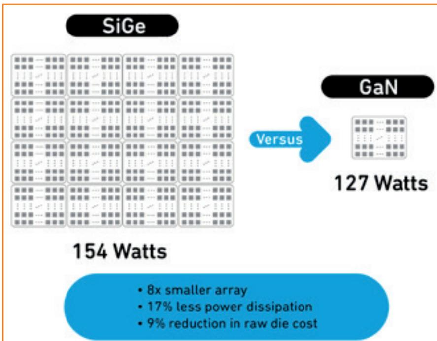
**Figure 5: Comparing an All-SiGe FWA system to a combination of SiGe beamforming with GaN front ends**
