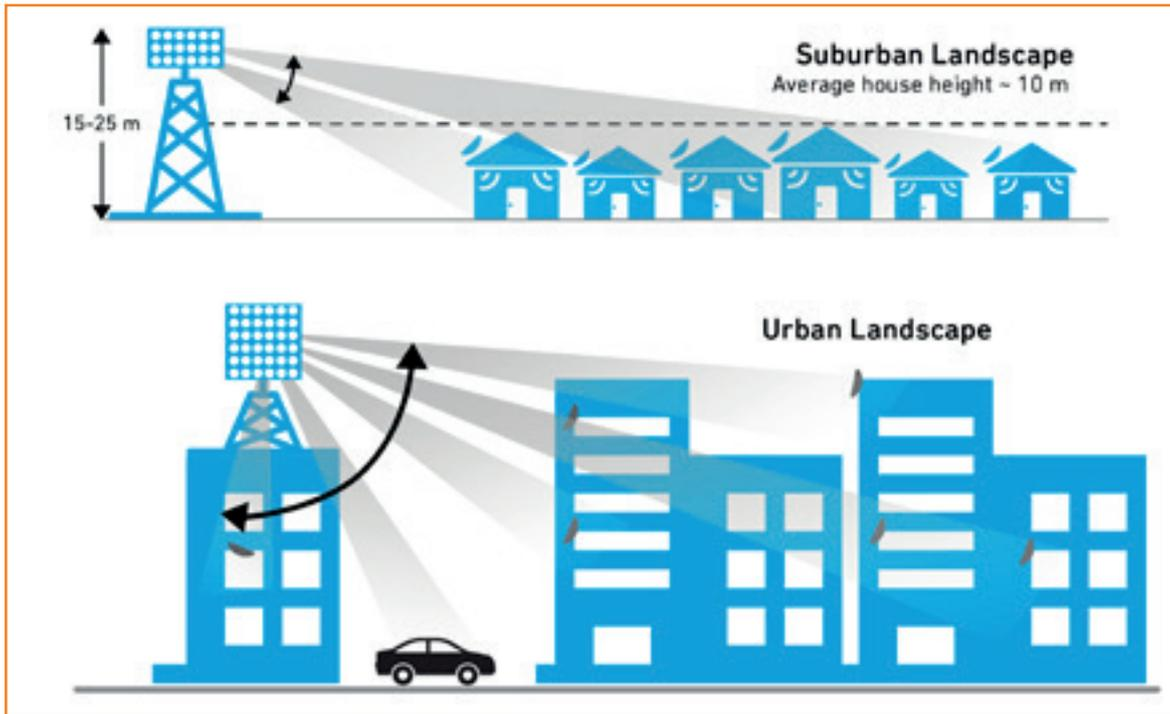
**Figure 1:** FWA array complexity depends upon the scanning range needed for the deployment scenario
