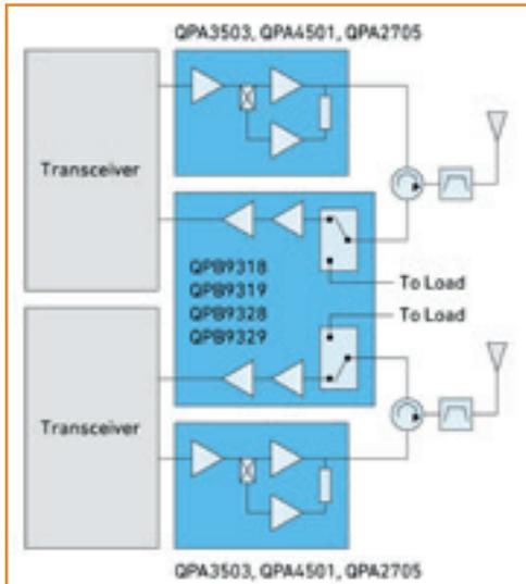
Figure 6: Qorvo FWA solutions: Sub-6GHz Massive MIMO GaN front ends
