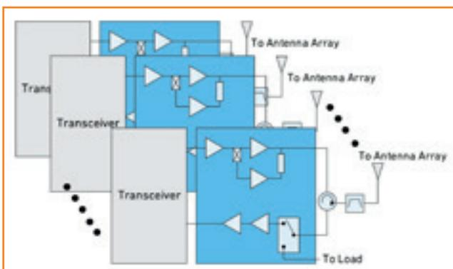
**Figure 2:** Integrated FEM with GaN Doherty PA and Switch-LNA
