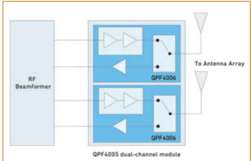
Figure 7: Qorvo FWA solutions: mmWave Massive MIMO GaN front ends
