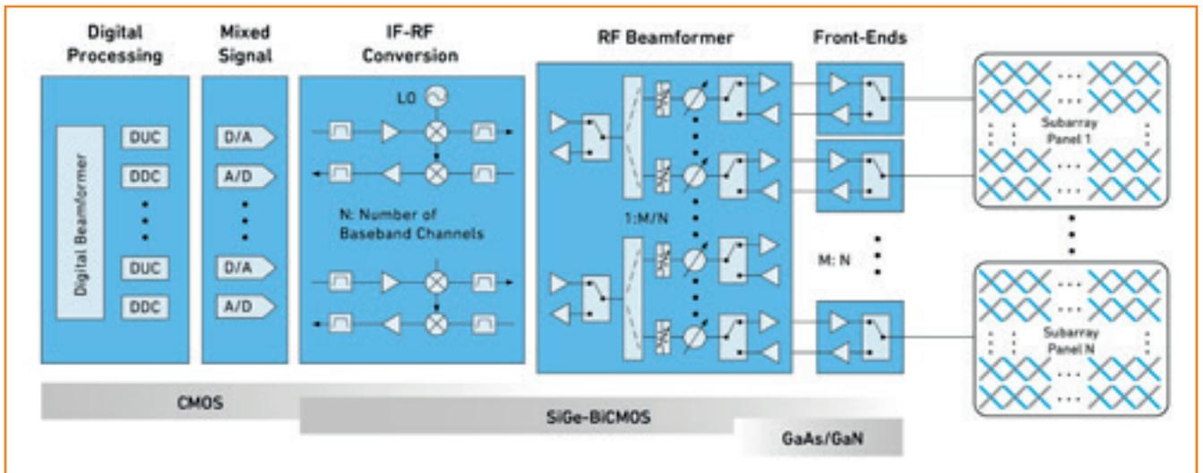
Figure 3: Hybrid beamforming Active Antenna Systems (AAS) block diagram
